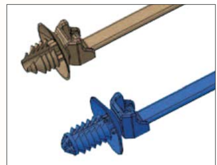
Example of re-engineering: 1-piece fixing tie. By optimising the lamella geometry, higher extraction forces can be achieved at lower push-in forces.
