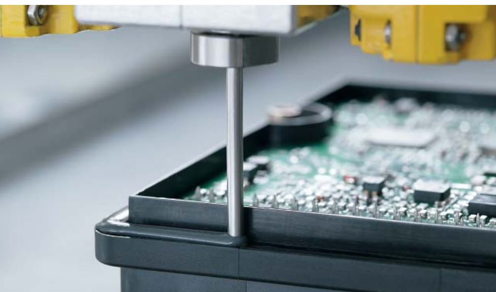
Automated bonding of housing components with WACKER silicones – reliable and efficient
